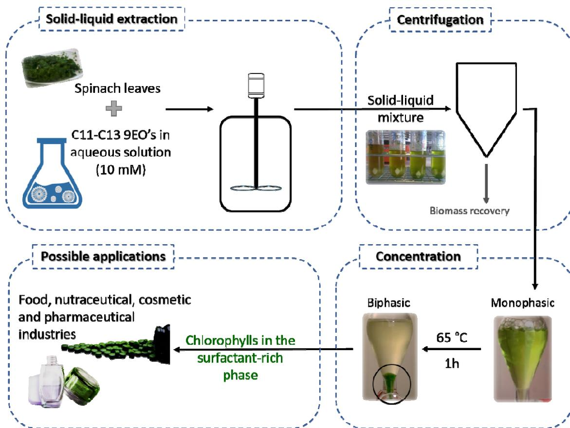
**Figure 8.** Scheme of the developed extraction-concentration process for chlorophylls from spinach leaves using aqueous solutions of non-ionic surfactants.
