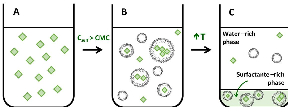
**Figure 2.** Schematic representation of the CPE. **A)** Initial aqueous solution containing a hydrophobic solute. **B)** Addition of non-ionic surfactants at a concentration higher than the CMC. **C)** Separation into two-phases by temperature changes.
