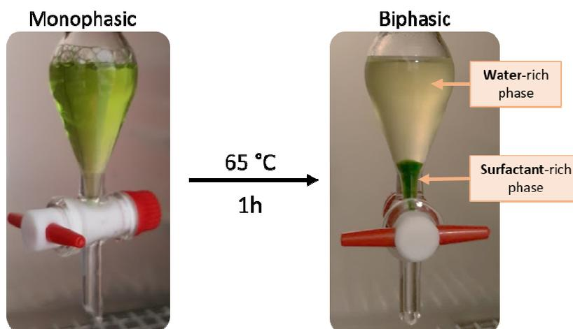
44 **Figure 6.** Scheme of the process used to concentrate chlorophylls.
